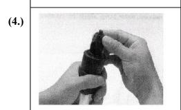
(4.) Insert part 6 into Gun Body's hexagon slot.
